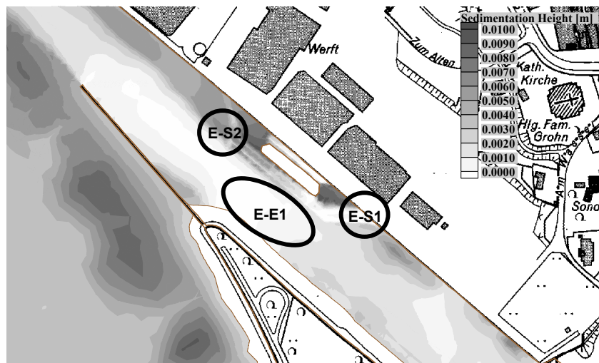
Figure 11: Sedimentation/Erosion during Ebb Period around/in the Sheet Piled Berth
