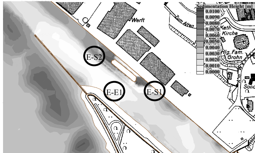
Fig. 9: Sedimentation/erosion during ebb period around/in the sheet piled berth.
