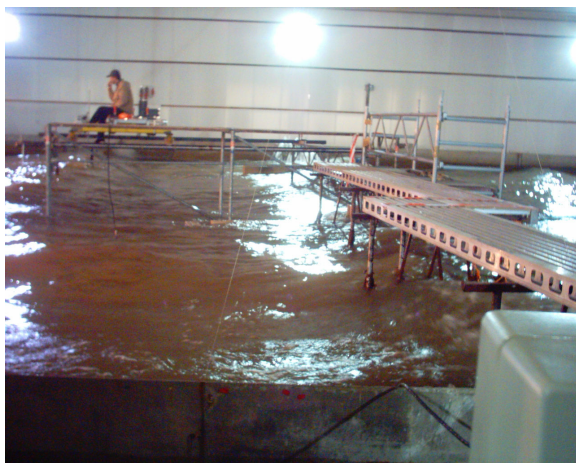
Figure 3-4: Sand Beach Deformation under Oblique Irregular Waves
