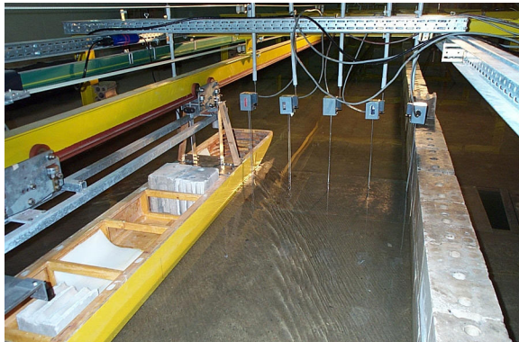
Figure 3-13: Ship Model at Supercritical Speed in RESTRICTED-WATER SHIP TOWING TANK MARIENWERDER
