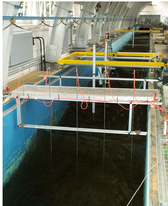
Figure 3-2: Tracer Release from Five Point Sources
