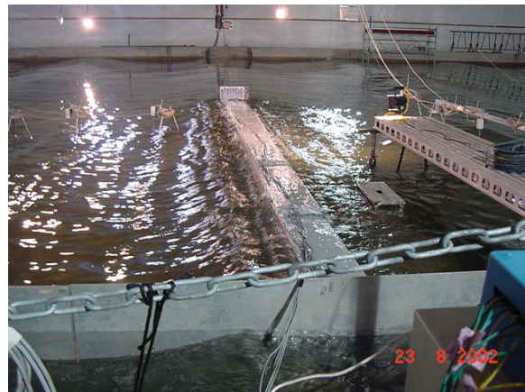
Figure 3-6: Floating Breakwater Model in 3-D WAVE BASIN MARIENWERDER under Non-Periodic Wave Attack
